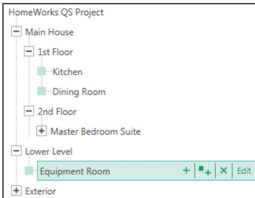
Use the Equipment toolbox to add a Specification Grade Dimming Panel to the area. If the dimming panel is not currently available in the toolbox, go to Edit Toolbox and add the dimming panel to the toolbox.
