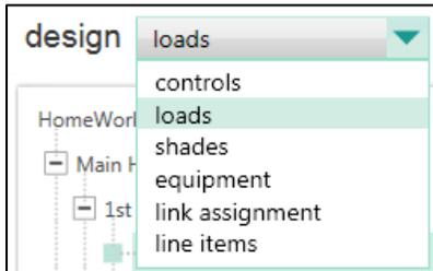
Upon selecting the option for the Load design screen, select an area that will contain the 0-10V loads by clicking on that area name in the tree to the left. The selected area will be highlighted green.
