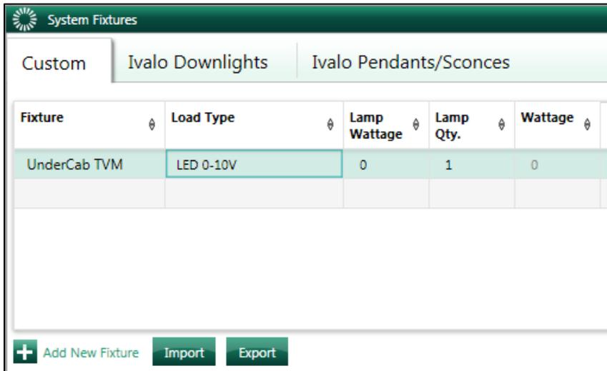
Click on Done to close the System Fixtures window and return to the Load Schedule for the selected area. Double-click in the Fixture field to reveal a drop-down menu with all currently created custom or Ivalo fixture options within the project. Select the 0-10V placeholder and the software will add a load schedule line item in the selected area for the 0-10V loads in that space.
