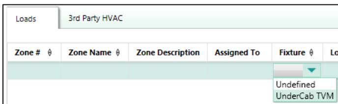
Provide a zone name, zone description, and any other pertinent field. Repeat this process for each 0-10V load that is to be controlled through a Specification Grade Panel output driving a TVM2.
