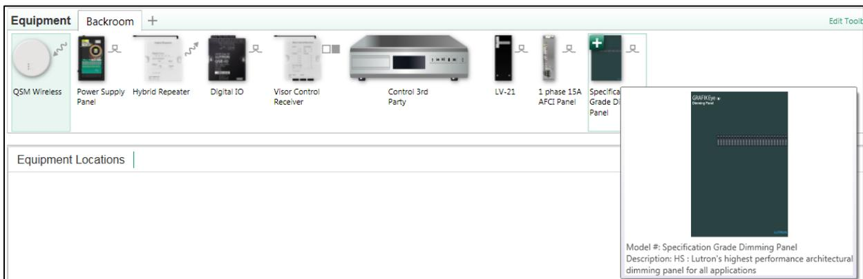
Configure the Specification Grade Dimming Panel in the software to match the needs of the application. A single panel can be configured to have a maximum of 144 zones. The physical size of the panel will vary based on the number of zones. The number of Specification Grade Panel Interfaces (SPIs), which link the dimming cards to the Processor, will also vary based on the zone count. A total of 6 SPIs would be required for the maximum panel size of 144 zones.
