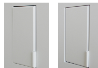
Correct: Dimmer/switch protrudes from faceplate. Incorrect: Dimmer/switch is flush with faceplate. Loosen control mounting screws.
