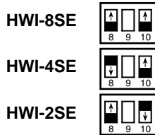
Figure 5: Factory Set DIP Switches (Do Not Modify)
