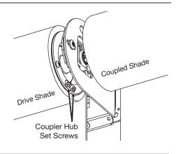
■ CAUTION: RISK OF FALLING OBJECTS. The Coupler Hub Set Screws are tightened at the factory to a torque of 6.0 in-lbs (0.7 N•m). Failure to re-tighten the Coupler Hub Set Screws to a torque of 6.0 in-lbs (0.7 N•m) could result in minor to moderate injury.
