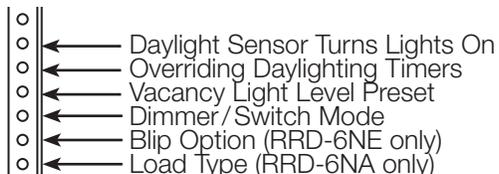
2. Press and release the tapswitch to select the feature for modification. Once the feature is selected the corresponding LED will flash.
