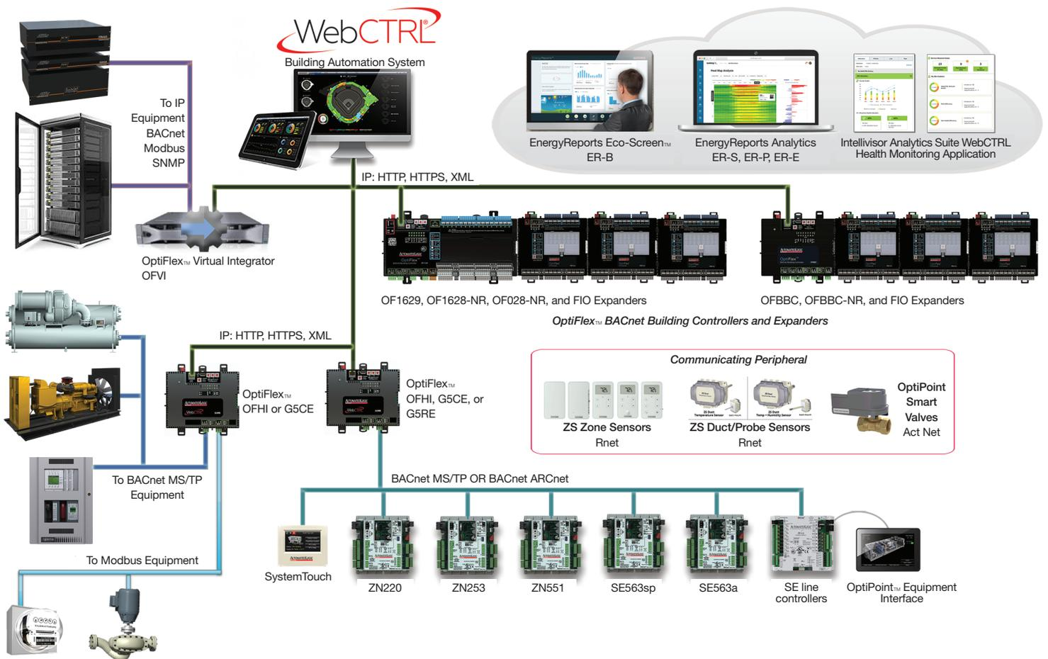
The WebCTRL® system’s open standards with BACnet native architecture makes integration with other mechanical and electrical building systems simple. BACnet is the global standard for open interoperability. The BACnet protocol is available as an American National Standard, a European standard, and global ISO Standard 16484-6:2014.
