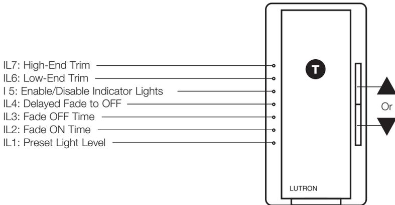
2. **To enter** the desired option, **press T**. Proceed to the specific programming option page to view programming instructions for desired option.
