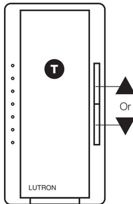
3. Press and release **T** to turn load OFF, then press **▲** once. If load does not turn ON or remains unstable, repeat Step 1 and in Step 2, increase light with **▲**.
