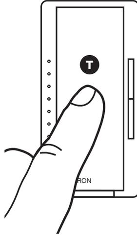
The default light setting has now been redefined. A single tap of **T** (when in *Normal Operation*, not *APM*) will now always return the dimmer to this selected light setting until preset is deactivated or reset. A double tap will always bring the lights to full intensity.
