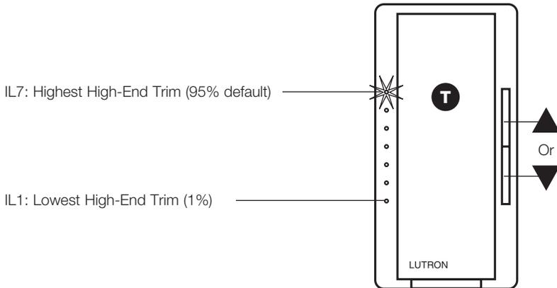
3. **To save** the desired *High-End Trim* setting, **press T**. This will exit out of the *High-End Trim* option and return to the *APM* main menu.
