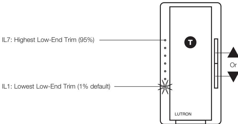
3. **To save** the desired *Low-End Trim* setting, **press T**. This will exit out of the *Low-End Trim* option and return to the *APM* main menu.
