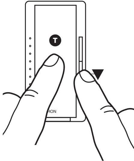
2. Press **▲** or **▼** to adjust light output until stable and not flickering. Press and release **T** to save setting.
