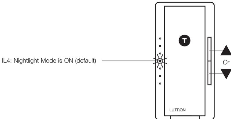
3. To save the desired *Enable/Disable Indicator Lights* setting, press **T**. This will exit out of the *Enable/Disable Indicator Lights* option and return to the *APM* main menu.
