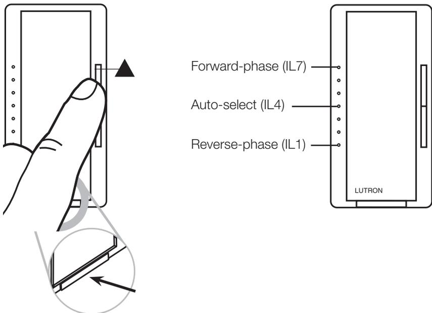
\* Phase auto-select defaults to reverse-phase unless the LED load cannot operate correctly. It will then switch to forward-phase automatically. Phase auto-select is only available when no neutral wire is connected.
