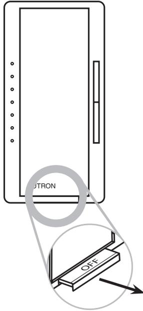
2. Press and hold **T**. While continuing to hold **T**, push the *FASS* to the *ON* position (in) and continue to hold **T** for approximately 5 seconds.
