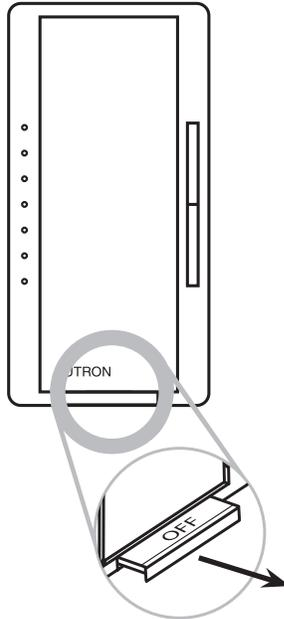
2. **Press and hold ▲. Close the FASS and continue to hold ▲ for 5 seconds.**
