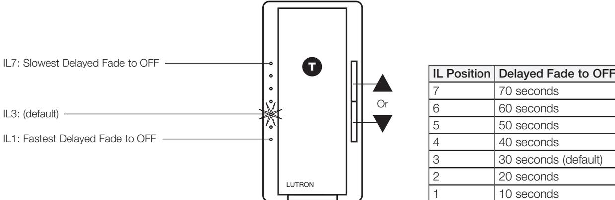
3. **To save** the desired *Delayed Fade to OFF*, press **T**. This will exit out of the *Delayed Fade to OFF* option and return to *APM* main menu.
