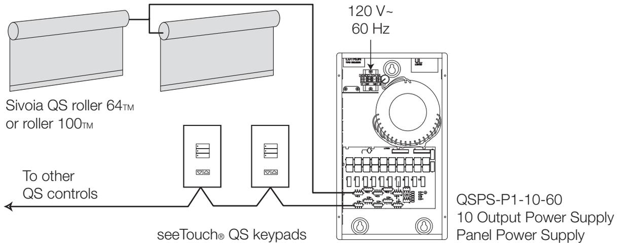
**Figure C** – Wiring diagram showing two drives daisy chained from one power output
