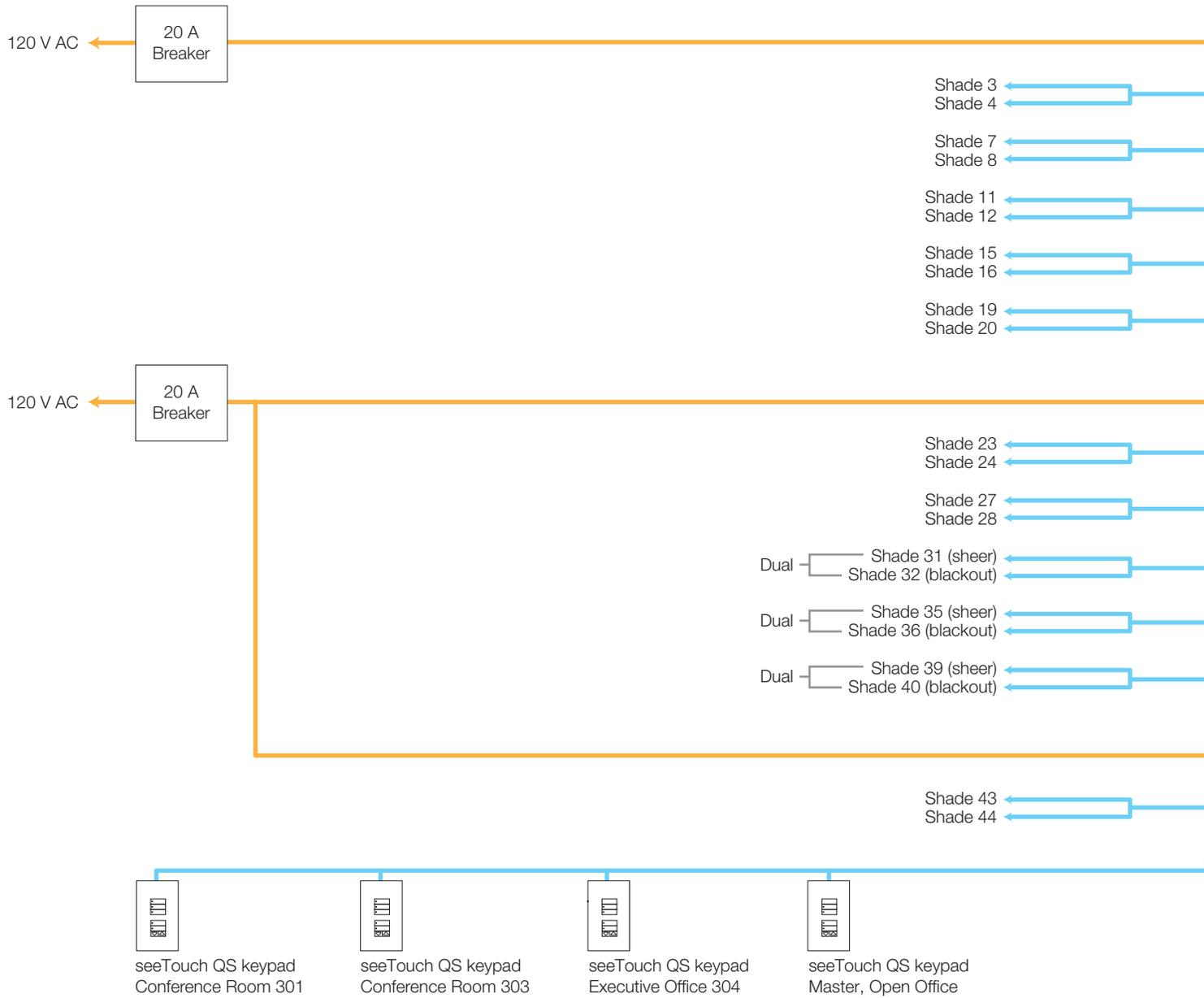
■ 4 Conductor Low Voltage Plenum Cable\* (communication link-shielded)
