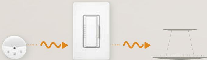
**How it works:** The daylight sensor sends a radio frequency signal to the dimmer “telling” it to brighten or dim the electric light based on the amount of daylight in the room. The dimmer, in turn, adjusts the amount of light emitted from the bulb in the light fixture.
