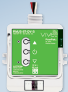
PowPak dimming module with 0-10V control
