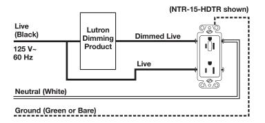
Top outlet will dim and bottom outlet is controlled by a switch.
