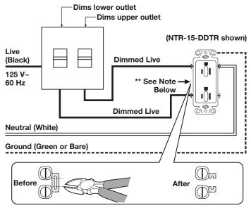
\*\* NOTE: To control each outlet of the receptacle independently, cut off the connecting link between the brass screws with a wire cutter.
