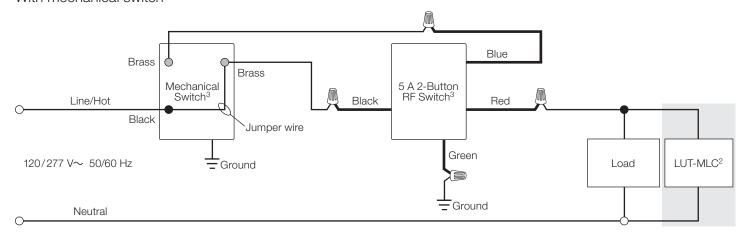
Multi-location Installation (for installations where 3 or more switches control the load)
