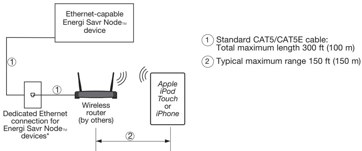
\* Energi Savr Node™ units are not designed to connect to an open network. Connection to an open network could result in reduced performance and Ethernet connectivity issues.
