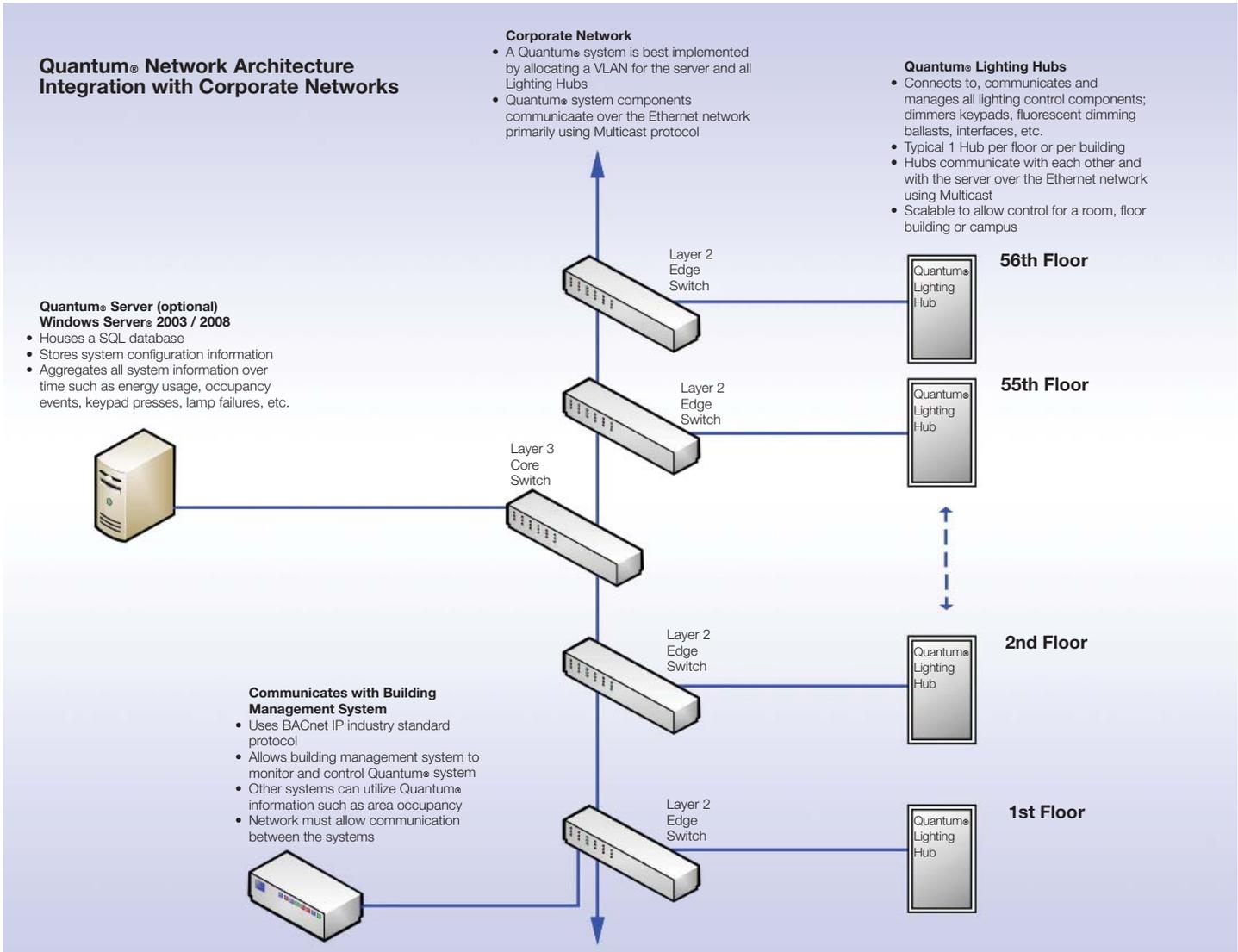
**Note:** The Quantum® server has no BACnet capabilities and thus has nothing to do with the BACnet connection. The BACnet stack exists in the embedded lighting control processors, and thus BACnet connectivity does not require a server running 24/7. Also, connecting to the server directly will NOT provide any BACnet information; the BMS connection must be made to the network on which the Quantum® lighting processors reside.
