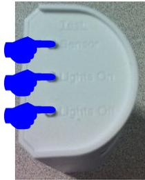
1. Remove the battery from the sensor and hold in the Sensor, Lights ON, and Lights OFF buttons.
