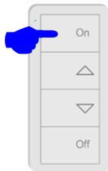
2. Press the top or bottom buttons to cycle through the 15 RF frequencies. Cycle through until you hear the Hybrid Repeater beep. Once you hear the beep, that means that the proper RF channel has been identified. At this point stop pressing any of the buttons that change the sensor's RF channel!
