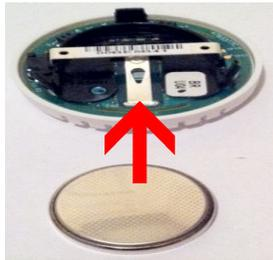
2. Continue to hold both buttons while sliding the battery back into place. After inserting the battery, continue holding both buttons for about 6 seconds until the LED flashes rapidly.
