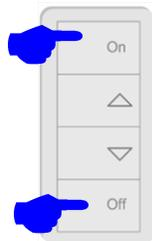
3. Press and hold the top and bottom buttons for at least 3 seconds to exit Frequency Changing Mode. The Hybrid Repeater will beep once the Pico successfully exits the Mode.
