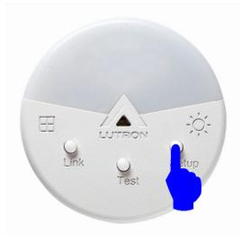
3. Press the Setup button to try the next RF channel (15 total). Press the Test button to repeat the current channel.
