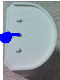
4. Continue to cycle through the RF channels until you hear the Hybrid Repeater beep. The beep indicates that the proper RF channel has been identified. At this point stop pressing any of the buttons that change the sensor's RF channel!
