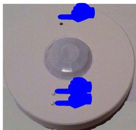
5. Hold in the Test, Lights ON, and Lights OFF buttons for about 3 seconds until the dome LED stops flashing.
