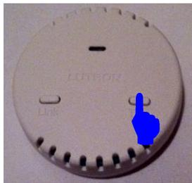
3. Press the Test button to try the next RF channel (15 total). Press the Link button to repeat the current channel.
