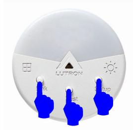
1. Remove the battery from the sensor and hold all three buttons.
