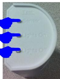
5. Hold in the Test, Lights ON, and Lights OFF buttons for about 3 seconds until the dome LED stops flashing.
