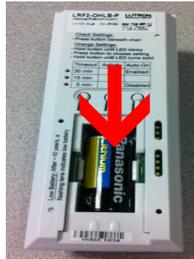
2. Continue to hold all three buttons while pressing the battery back into place. After inserting the battery, continue holding all three buttons for about 3 seconds until the LED flashes rapidly.
