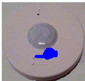
4. Continue to cycle through the RF channels until you hear the Hybrid Repeater beep. The beep indicates that the proper RF channel has been identified. At this point stop pressing any of the buttons that change the sensor's RF channel!
