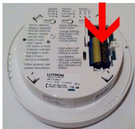
2. Continue to hold all three buttons while pushing the battery back into place. After inserting the battery, continue holding the three buttons for about 3 seconds until the dome LED flashes rapidly.
