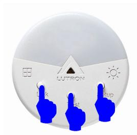
5. Hold all three buttons for about 6 seconds until the LED stops flashing.
