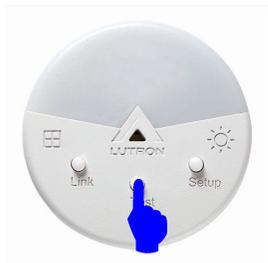
4. Continue to cycle through the RF channels until you hear the QSM beep. The beep indicates that the proper RF channel has been identified. At this point stop pressing any of the buttons that change the sensor's RF channel!
