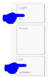
3. Press and hold the On/Open (top) and Off/Close (bottom) buttons for at least 3 seconds to exit Frequency Changing Mode. The Hybrid Repeater will beep once the Pico successfully exits the Mode.
