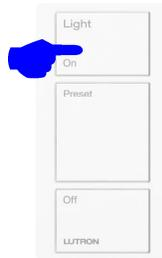
1. Triple tap and hold the On/Open button (top button) of the Pico. Hold the button for at least 15 seconds. The Hybrid Repeater will beep to let you know that the Pico is now in Frequency Changing Mode.
