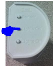
3. Press the LIGHTS ON button to try the next RF channel (15 total). Press the LIGHTS OFF button to try the previous RF channel. Press the TEST button to repeat the current channel.
