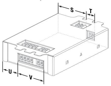
S 1.38 in (35 mm) T 0.64 in (16 mm) U 0.88 in (22 mm) V 1.53 in (39 mm)
