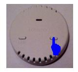
4. Continue to cycle through the RF channels until you hear the Main or Aux Repeater beep. The beep indicates that the proper RF channel has been identified. At this point stop pressing any of the buttons that change the sensor's RF channel!
