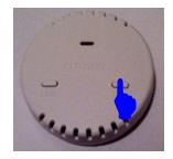
3. Press the Test button to try the next RF channel (15 total). Press the Link button to repeat the current channel.
