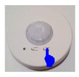
5. Continue to cycle through the RF channels until you hear the Main or Aux Repeater beep. The beep indicates that the proper RF channel has been identified. At this point stop pressing any of the buttons that change the sensor's RF channel!
