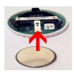
2. Continue to hold both buttons while sliding the battery back into place. After inserting the battery, continue holding both buttons for about 6 seconds until the LED flashes rapidly.
