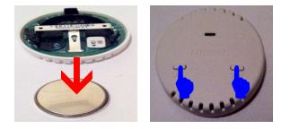
1. Remove the battery from the sensor and hold in the Test and Link buttons.
