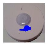
3. Press the Lights ON button to try the next RF channel (15 total). Press the Lights OFF button to try the previous channel. Press the Test button to repeat the current channel.
