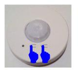
6. Hold in the P Button and Test button For 6 seconds until the dome LED stops rapid flashing.
