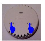
5. Hold in the Test and Link buttons for about6 seconds until the LED stops flashing.
