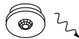
LRF2-OCR2B-P-WH 434MHZ WIRELESS OCCUPANCY/VACANCY SENSOR 3.57"[90,7mm] (DIA) X 1.13"[28,7mm] (D) *DEVICE IS SURFACE-MOUNTED AND BATTERY POWERED, DOES NOT REQUIRE POWER FEED
