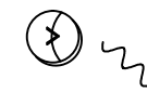
LRF2-DCRB-WH 434MHZ WIRELESS DAYLIGHT SENSOR 1.6"[40,6mm] (DIA) X 0.7"[17,8mm] (D) *DEVICE IS SURFACE-MOUNTED AND BATTERY POWERED, DOES NOT REQUIRE POWER FEED
