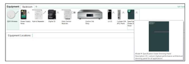
Configure the Specification Grade Dimming Panel in the software to match the needs of the application. A single panel can be configured to have a maximum of 144 zones. The physical size of the panel will vary based on the number of zones. The number of Specification Grade Panel Interfaces (SPIs), which link the dimming cards to the Processor, will also vary based on the zone count. A total of 6 SPIs would be required for the maximum panel size of 144 zones.
