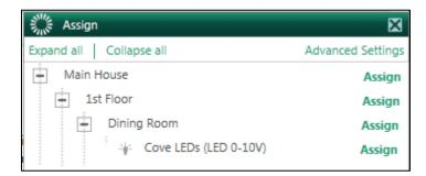
The zone will now be assigned to the selected output on the panel. A TVI should appear in the *Interface* field.
