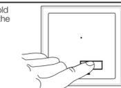
**2** Add the Sensor to the Switch by pressing and holding the "Lights Off" button on the front of the Sensor for approximately 6 seconds until the lens flashes briefly. The lights in the room will also flash 3 times, indicating the Sensor has been successfully added. The Switch will exit set-up mode automatically.
