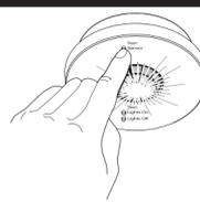
**NOTE:** There is a warm-up period of approximately 40 seconds after the batteries are installed before the test mode can be activated. If the button is pressed during this time, the lens will flash continuously until the warm-up period is complete, and then the test mode will be automatically entered.
