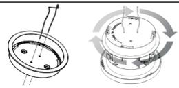
**1.2** Mount Sensor to a ceiling tile by inserting the wire legs through the tile, making sure the Sensor is flush to the tile.
