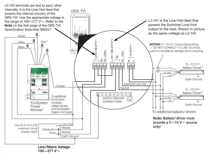
1 The red wire is not used. Cap off the red wire using a wire connector. Do not wire the red wire to ground or to any other wiring.
