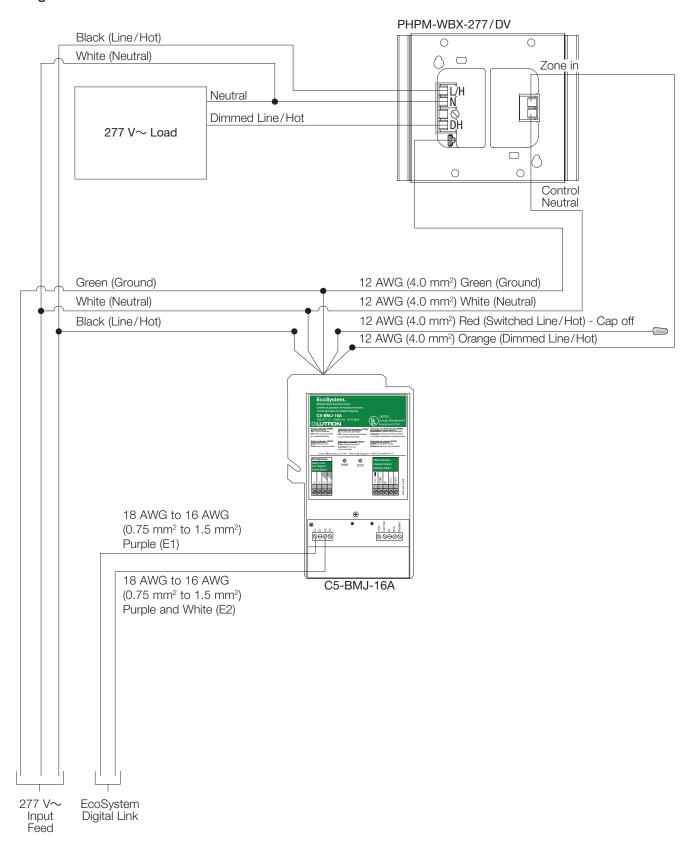
Separate Power Feeds for Control and Load: 120  $V\sim$  Control Voltage
