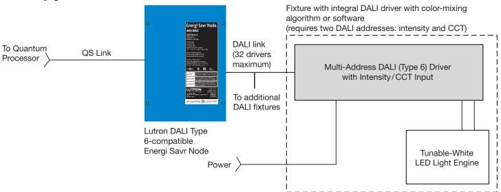
Figure 18: DALI Type 6 implementation providing independent control of intensity and color temperature.
