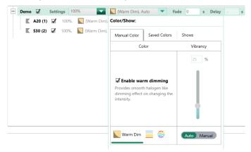
Figure 6: Available dim-to-warm emulations available with Ketra lamps.
