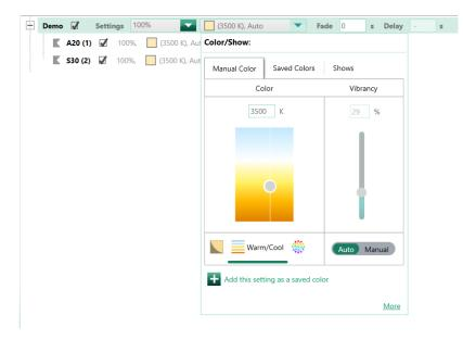
Figure 20: Ketra not only allows independent control of intensity and CCT, but also allows a user to adjust vibrancy (maintaining CCT while adjusting the spectral power density to manipulate color reflection in the space).
