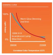
Figure 3: CCT curves for incandescent lamp and USAI Lighting luminaire with Warm Glow<sub>®</sub> Dimming technology.
