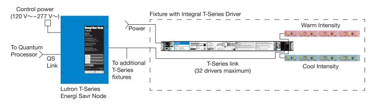
Figure 13: Lutron T-Series control and driver providing independent control of intensity and color temperature.
