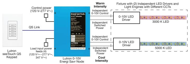
Figure 7: Lutron 0-10V Energi Savr Node unit controlling two independent LED drivers in a tunable white application (NOT RECOMMENDED)
