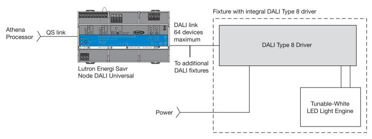
Figure 19: DALI Type 8 implementation providing independent control of intensity and color temperature
