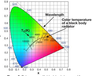
Figure 2: Color space with black body locus and lines of constant color temperature ( $T_c$ ).
