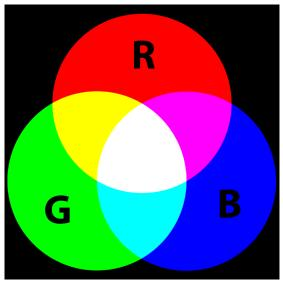
Figure 22: RGB additive color mixing.
