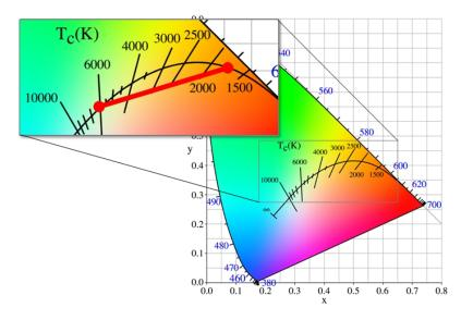
**Figure 9:** Using single colors (warm and cool) to achieve color tuning will cause colors in between the two extremes to deviate from the black body locus.
