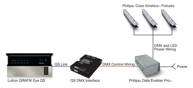
Figure 23: Lutron GRAFIK Eye QS unit controlling Philips₀ Color Kinetics™ fixtures through DMX control.
