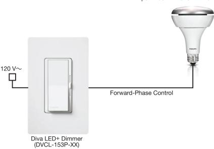
Philips BR30 DimTone<sub>®</sub> with dim-to-warm LED
