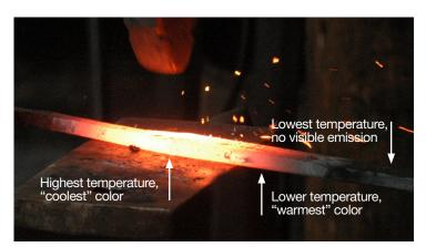
Figure 1: Heated piece of iron showing the black body color temperatures.
