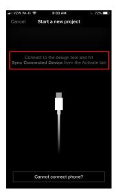
Selecting this option will prompt you to press the **Sync Connected Device** in the software. Once synchronizing is complete, the app will display a summary of the current activation status and the area tree for the project. This is reflective of all active Ketra loads in the project.
