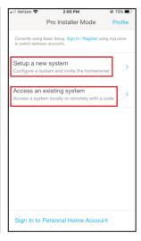
Once the **Profile** information has been entered, back out of this screen using the < icon and return to the main **Pro Installer** menu. Tap on **Setup a new system** to begin setting up a new system. On the next screen choose **HomeWorks** as the system option and follow the prompts. In order to finalize the setup, the button on the QSX processor will need to be pressed to prove physical access.
