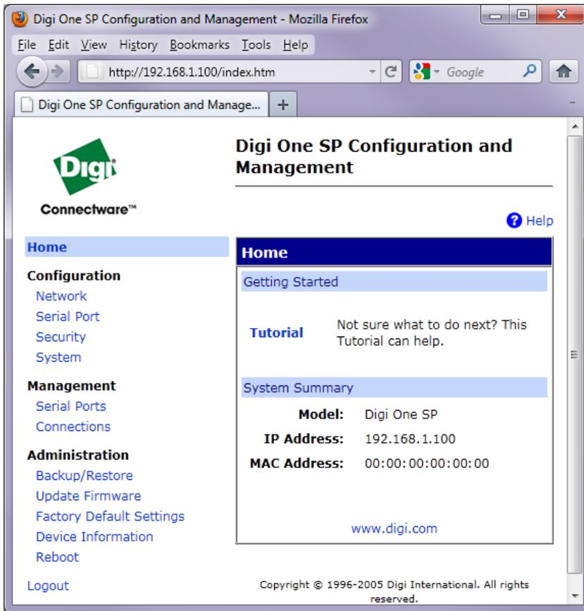
3. Configure the network settings on the Ethernet to RS-232 converter device by clicking on the "Network" option on the left side. It is recommended to use a static IP address. This address should be outside the DHCP range of the router. The device must be on the same network and subnet as the HWQS processor. Be sure to Apply the settings. The device may need to reboot for the settings to take effect.
