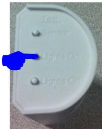
3. Press the LIGHTS ON button to try the next RF channel (15 total). Press the LIGHTS OFF button to try the previous RF channel. Press the TEST button to repeat the current channel.
