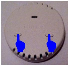
1. Remove the battery from the sensor and hold in the Test and Link buttons.
