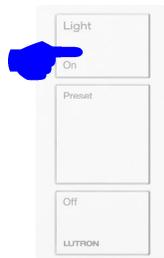
1. Triple tap and hold the On/Open button (top button) of the Pico. Hold the button for at least 15 seconds. The Main and Aux Repeaters will beep to let you know that the Pico is now in Frequency Changing Mode.
