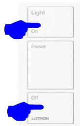
3. Press and hold the On/Open (top) and Off/Close (bottom) buttons for at least 3 seconds to exit Frequency Changing Mode. The Main and Aux Repeaters will beep once the Pico successfully exits the Mode.
