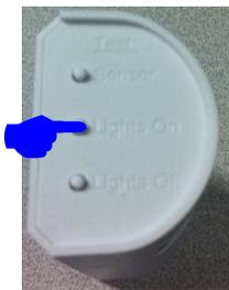
4. Continue to cycle through the RF channels until you hear the Main or Aux Repeater beep. The beep indicates that the proper RF channel has been identified. At this point stop pressing any of the buttons that change the sensor's RF channel!
