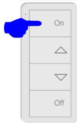
2. Press the top or bottom buttons to cycle through the 15 RF frequencies. Cycle through until you hear the Main or Aux Repeaters beep. Once you hear the beep, that means that the proper RF channel has been identified. At this point stop pressing any of the buttons that change the sensor's RF channel!
