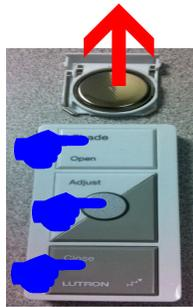
1. Remove the battery from the Pico and hold in the Open/On, Preset, and Close/Off buttons.
