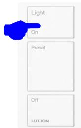
2. Press the On/Open (top) or Off/Close (bottom) buttons to cycle through the 15 RF frequencies. Cycle through until you hear the Main or Aux Repeaters beep. Once you hear the beep, that means that the proper RF channel has been identified. At this point stop pressing any of the buttons that change the sensor's RF channel!
