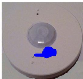
4. Continue to cycle through the RF channels until you hear the Main or Aux Repeater beep. The beep indicates that the proper RF channel has been identified. At this point stop pressing any of the buttons that change the sensor's RF channel!
