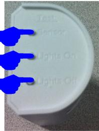
1. Remove the battery from the sensor and hold in the Sensor, Lights ON, and Lights OFF buttons.
