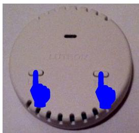
5. Hold in the Test and Link buttons for about 6 seconds until the LED stops flashing.
