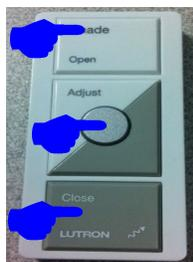
5. Hold in the Open/On, Preset, and Close/Off buttons for about 3 seconds until the LED stops flashing.
