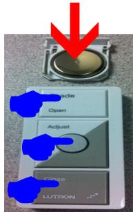
2. Continue to hold all three buttons while pressing the battery back into place. After inserting the battery, continue holding all three buttons for about 3 seconds until the LED flashes about once per second.
