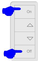
3. Press and hold the top and bottom buttons for at least 3 seconds to exit Frequency Changing Mode. The Main and Aux Repeaters will beep once the Pico successfully exits the Mode.
