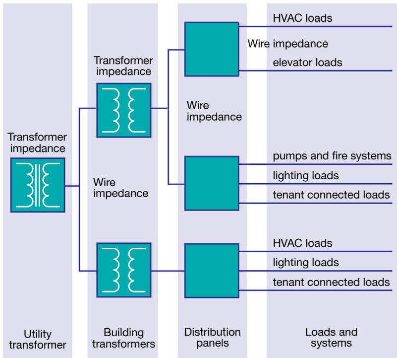
**Figure 5 – Building Power Distribution System**
