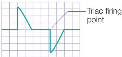
**Figure 3 – Triac Conduction Time**
