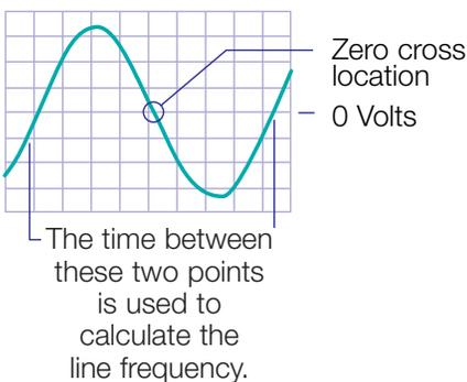
**Figure 4 – Zero Cross and Line Frequency**
