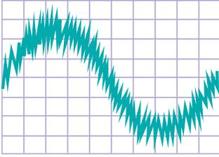
**Figure 6 – High Frequency Noise >5kHz**
