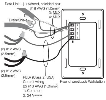
Note: Use appropriate wire connecting devices as specified by local codes.
