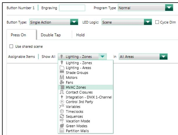
After the button has been configured, select HVAC zones from the Assignable Items drop down menu. Find the zone that you would like to add to the button and roll your cursor over top of the checkbox to the right of the zone name. Select the parameters that need to change based on
