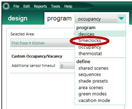
Create a new Timeclock event, setting the name, days of week, and time of the event. On the right hand side, select the Program Type. Select the HVAC zones to be affected by the event. Timeclock events can be used to adjust setpoints, operating modes, and fan speeds.
