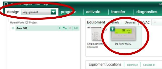
Once the 3<sup>rd</sup> Party HVAC control has been added to the **Equipment Locations** area, provide a name for the HVAC control and select **Lutron Thermostat** as the Manufacturer. Note: when adding the 3<sup>rd</sup> Party HVAC interface, a zone is automatically added by default. All zones should be created as seen in the previous section and this auto-created zone can be deleted.
